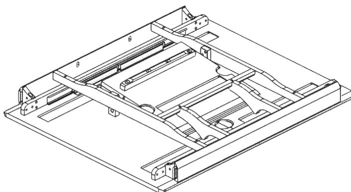
2. Slot the two leg rails into the ends of the table as shown below.
