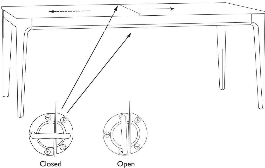
5. The two leaves are held closed by two keepers (above), one on either side of the underside of the table where the join is. Turn the bar on them to release the leaves then, as they are reciprocal, gently pull open one leaf, as far as it will go and the other will automatically open with it.
