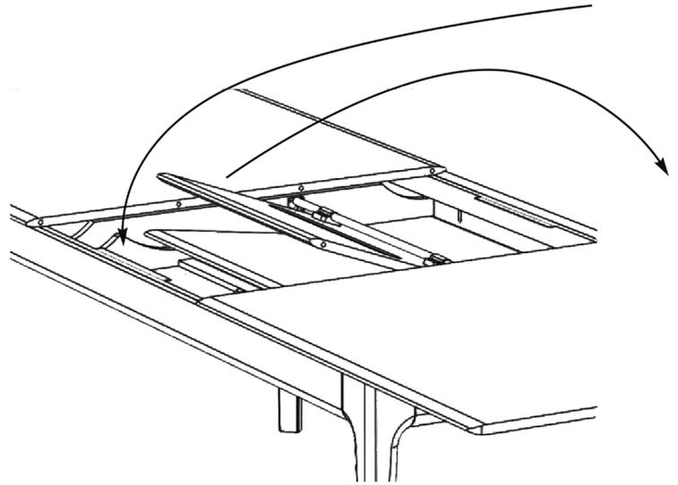
6. Lift the top flap of the butterfly extension leaves and pull it up and back over the table top as shown in the following 3 stages. As you open it the lower leaf will glide over the ramp and up into place.
