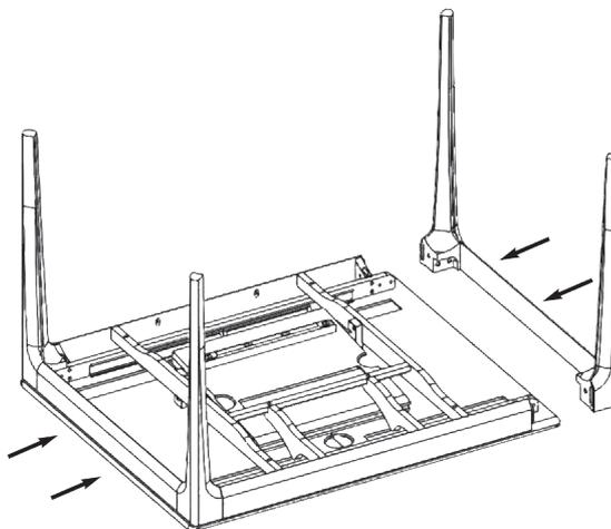
3. Using the Allen key provided screw a bolt into the single hole first, then screw a bolt into each of the two pre drilled holes on the other side of the leg, as shown below.
