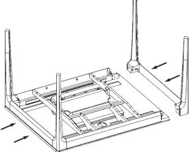
3. Using the Allen key provided screw a bolt into the single hole first, then screw a bolt into each of the two pre drilled holes on the other side of the leg, as shown below.
